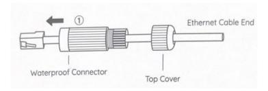
2. Put the rubber seal ring around the Ethernet cable between the top cover and the waterproof connector.
