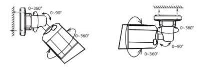
Point the camera at the desired location and use the screws provided to mount it.
